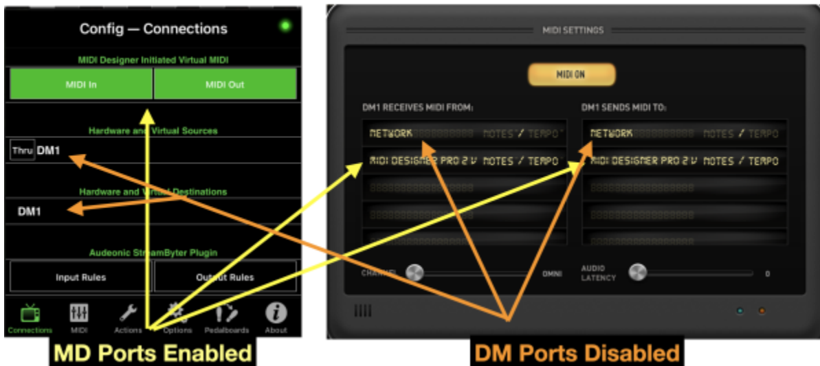
Virtual connection between MD and DM1 on iPad MD virtual connections enabled, DM1 disabled DM1 identifies its virtual ports as "network."
